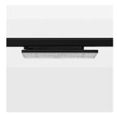
Surface-mounted luminaire with LED, rated life of the LED L90/B50 50000 h (tambient 25°C), colour rendering index CRI > 80, chromaticity tolerance 3 SDCM (initial), wide, homogeneous light distribution pattern 30°, TIR-lens made of PMMA, luminaire housing sheet steel, powder-coated, black, locking mechanism to aligned in 15° steps, rotation angle 300°, In-Track-Adapter, On/Off, 220-240 V~ / 50-60 Hz, max. 27 luminaires per circuit (B16A fuse)
