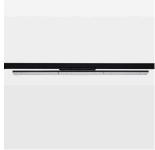
Surface-mounted luminaire with LED, rated life of the LED L90/B50 50000 h (tambient 25°C), colour rendering index CRI > 80, chromaticity tolerance 3 SDCM (initial), wide, homogeneous light distribution pattern (60°), TIR-lens made of PMMA, luminaire housing sheet steel, powder-coated, black, locking mechanism to aligned in 15° steps, rotation angle 300°, In-Track-Adapter, On/Off, 220-240 V~ / 50-60 Hz
