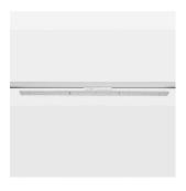
Surface-mounted luminaire with LED, rated life of the LED L90/B50 50000 h (tambient 25°C), colour rendering index CRI > 80, chromaticity tolerance 3 SDCM (initial), wide, homogeneous light distribution pattern 30°, TIR-lens made of PMMA, luminaire housing sheet steel, powder-coated, white, locking mechanism to aligned in 15° steps, rotation angle 300°, In-Track-Adapter, On/Off, 220-240 V~ / 50-60 Hz
