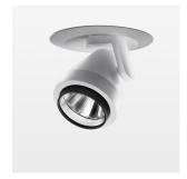
Semi-recessed luminaire with LED, rated life of the LED L80/B10 50000 h (tambient 25°C), colour rendering index CRI > 96, chromaticity tolerance 2 SDCM (initial), rotation-symmetrical reflector with circular light distribution pattern, reflector pure aluminium 99,99% in MIRO-Silver®, segmented and faceted, 3D lens silicon to reduce the proportion of scattered light, die-cast aluminium, powder-coated, rotation angle 400°, swivel angle +/- 85°, white, separate driver unit
