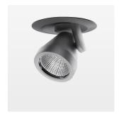
Semi-recessed luminaire with LED, rated life of the LED L80/B10 50000 h (tambient 25°C), colour rendering index CRI > 96, chromaticity tolerance 2 SDCM (initial), rotation-symmetrical reflector with circular light distribution pattern, reflector pure aluminium 99,99% in MIRO-Silver®, segmented and faceted, 3D lens silicon to reduce the proportion of scattered light, die-cast aluminium, powder-coated, rotation angle 400°, swivel angle +/- 85°, silver, separate driver unit
