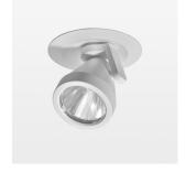
Semi-recessed luminaire with LED, rated life of the LED L80/B10 50000 h (tambient 25°C), colour rendering index CRI > 95, chromaticity tolerance 2 SDCM (initial), rotation-symmetrical reflector with circular light distribution pattern, reflector pure aluminium 99,99% in MIRO-Silver®, segmented and faceted, 3D lens silicon to reduce the proportion of scattered light, die-cast aluminium, powder-coated, rotation angle 400°, swivel angle +/- 85°, white, separate driver unit
