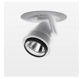
Semi-recessed luminaire with LED, rated life of the LED L80/B10 50000 h (tambient 25°C), colour rendering index CRI > 96, chromaticity tolerance 2 SDCM (initial), rotation-symmetrical reflector with circular light distribution pattern, reflector pure aluminium 99,99% in MIRO-Silver®, segmented and faceted, 3D lens silicon to reduce the proportion of scattered light, die-cast aluminium, powder-coated, rotation angle 400°, swivel angle +/- 85°, white, separate driver unit
