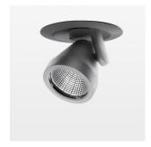
Semi-recessed luminaire with LED, rated life of the LED L80/B10 50000 h (tambient 25°C), colour rendering index CRI > 96, chromaticity tolerance 2 SDCM (initial), rotation-symmetrical reflector with circular light distribution pattern, reflector pure aluminium 99,99% in MIRO-Silver®, segmented and faceted, 3D lens silicon to reduce the proportion of scattered light, die-cast aluminium, powder-coated, rotation angle 400°, swivel angle +/- 85°, silver, separate driver unit
