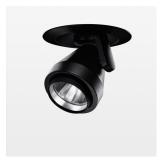
Semi-recessed luminaire with LED, rated life of the LED L80/B10 50000 h (tambient 25°C), colour rendering index CRI > 96, chromaticity tolerance 2 SDCM (initial), rotation-symmetrical reflector with circular light distribution pattern, reflector pure aluminium 99,99% in MIRO-Silver®, segmented and faceted, 3D lens silicon to reduce the proportion of scattered light, die-cast aluminium, powder-coated, rotation angle 400°, swivel angle +/- 85°, black, separate driver unit
