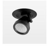
Semi-recessed luminaire with LED, rated life of the LED L80/B10 50000 h (tambient 25°C), colour rendering index CRI > 90, chromaticity tolerance 2 SDCM (initial), reflector with circular light distribution pattern, reflector pure aluminium 99,99% in MIRO-Silver®, segmented and faceted, 3D lens silicon to reduce the proportion of scattered light, die-cast aluminium, powder-coated, rotation angle 400°, swivel angle +/- 85°, black, separate driver unit
