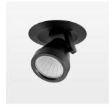
Semi-recessed luminaire with LED, rated life of the LED L80/B10 50000 h (tambient 25°C), colour rendering index CRI > 90, chromaticity tolerance 2 SDCM (initial), reflector with circular light distribution pattern, reflector pure aluminium 99,99% in MIRO-Silver®, segmented and faceted, die-cast aluminium, powder-coated, rotation angle 400°, swivel angle +/- 85°, black, potentiometer to adjust the brightness, separate driver unit
