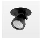
Semi-recessed luminaire with LED, rated life of the LED L80/B10 50000 h (tambient 25°C), colour rendering index CRI > 96, chromaticity tolerance 2 SDCM (initial), reflector with circular light distribution pattern, reflector pure aluminium 99,99% in MIRO-Silver®, segmented and faceted, 3D lens silicon to reduce the proportion of scattered light, die-cast aluminium, powder-coated, rotation angle 400°, swivel angle +/- 85°, black, separate driver unit
