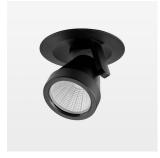
Semi-recessed luminaire with LED, rated life of the LED L80/B10 50000 h (tambient 25°C), colour rendering index CRI > 80, chromaticity tolerance 2 SDCM (initial), reflector with circular light distribution pattern, reflector pure aluminium 99,99% in MIRO-Silver®, segmented and faceted, 3D lens silicon to reduce the proportion of scattered light, die-cast aluminium, powder-coated, rotation angle 400°, swivel angle +/- 85°, black, potentiometer to adjust the brightness, separate driver unit
