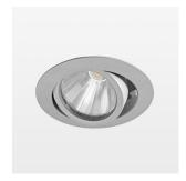
Recessed luminaire with LED, rated life of the LED L80/B10 50000 h (tambient 25°C), colour rendering index CRI > 80, chromaticity tolerance 3 SDCM (initial), rotation-symmetrical reflector with circular light distribution pattern, reflector pure aluminium 99,99% in MIRO-Silver®, segmented and faceted, 3D lens silicon to reduce the proportion of scattered light, die-cast aluminium, powder-coated, rotation angle, swivel angle +/- 25°, silver,
