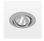
Recessed luminaire with LED, rated life of the LED L80/B10 50000 h (tambient 25°C), colour rendering index CRI > 90, chromaticity tolerance 3 SDCM (initial), rotation-symmetrical reflector with circular light distribution pattern, reflector pure aluminium 99,99% in MIRO-Silver®, segmented and faceted, 3D lens silicon to reduce the proportion of scattered light, die-cast aluminium, powder-coated, rotation angle, swivel angle +/- 25°, silver,
