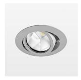
Recessed luminaire with LED, rated life of the LED L80/B10 50000 h (tambient 25°C), colour rendering index CRI > 80, chromaticity tolerance 2 SDCM (initial), reflector with oval light distribution pattern, reflector pure aluminium 99,99% in MIRO-Silver®, segmented, die-cast aluminium, powdercoated, rotation angle, swivel angle +/- 25°, silver,
