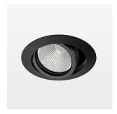
Recessed luminaire with LED, rated life of the LED L80/B10 50000 h (tambient 25°C), colour rendering index CRI > 80, chromaticity tolerance 2 SDCM (initial), reflector with circular light distribution pattern, reflector pure aluminium 99,99% in MIRO-Silver®, segmented and faceted, die-cast aluminium, powder-coated, rotation angle, swivel angle +/- 25°, black,
