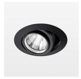
Recessed luminaire with LED, rated life of the LED L80/B10 50000 h (tambient 25°C), colour rendering index CRI > 90, chromaticity tolerance 2 SDCM (initial), rotation-symmetrical reflector with circular light distribution pattern, reflector pure aluminium 99,99% in MIRO-Silver®, segmented and faceted, 3D lens silicon to reduce the proportion of scattered light, die-cast aluminium, powder-coated, rotation angle, swivel angle +/- 25°, black,
