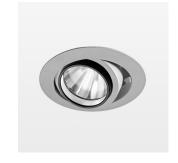
Recessed luminaire with LED, rated life of the LED L80/B10 50000 h (tambient 25°C), colour rendering index CRI > 96, chromaticity tolerance 2 SDCM (initial), rotation-symmetrical reflector with circular light distribution pattern, reflector pure aluminium 99,99% in MIRO-Silver®, segmented and faceted, 3D lens silicon to reduce the proportion of scattered light, die-cast aluminium, powder-coated, rotation angle, swivel angle +/- 25°, silver,
