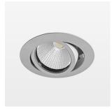
Recessed luminaire with LED, rated life of the LED L80/B10 50000 h (tambient 25°C), colour rendering index CRI > 80, chromaticity tolerance 2 SDCM (initial), reflector with circular light distribution pattern, reflector pure aluminium 99,99% in MIRO-Silver®, segmented and faceted, die-cast aluminium, powder-coated, rotation angle, swivel angle +/- 25°, silver,
