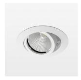
Recessed luminaire with LED, rated life of the LED L80/B10 50000 h (tambient 25°C), colour rendering index CRI > 90, chromaticity tolerance 2 SDCM (initial), reflector with circular light distribution pattern, reflector pure aluminium 99,99% in MIRO-Silver®, segmented and faceted, 3D lens silicon to reduce the proportion of scattered light, die-cast aluminium, powder-coated, rotation angle, swivel angle +/- 25°, white,
