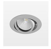
Recessed luminaire with LED, rated life of the LED L80/B10 50000 h (tambient 25°C), colour rendering index CRI > 90, chromaticity tolerance 2 SDCM (initial), reflector with circular light distribution pattern, reflector pure aluminium 99,99% in MIRO-Silver®, segmented and faceted, 3D lens silicon to reduce the proportion of scattered light, die-cast aluminium, powder-coated, rotation angle, swivel angle +/- 25°, silver,
