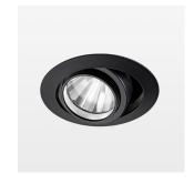
Recessed luminaire with LED, rated life of the LED L80/B10 50000 h (tambient 25°C), colour rendering index CRI > 80, chromaticity tolerance 2 SDCM (initial), rotation-symmetrical reflector with circular light distribution pattern, reflector pure aluminium 99,99% in MIRO-Silver®, segmented and faceted, 3D lens silicon to reduce the proportion of scattered light, die-cast aluminium, powder-coated, rotation angle, swivel angle +/- 25°, black,
