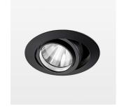
Recessed luminaire with LED, rated life of the LED L80/B10 50000 h (tambient 25°C), colour rendering index CRI > 96, chromaticity tolerance 2 SDCM (initial), rotation-symmetrical reflector with circular light distribution pattern, reflector pure aluminium 99,99% in MIRO-Silver®, segmented and faceted, 3D lens silicon to reduce the proportion of scattered light, die-cast aluminium, powder-coated, rotation angle, swivel angle +/- 25°, black,
