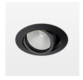
Recessed luminaire with LED, rated life of the LED L80/B10 50000 h (tambient 25°C), colour rendering index CRI > 90, chromaticity tolerance 2 SDCM (initial), reflector with circular light distribution pattern, reflector pure aluminium 99,99% in MIRO-Silver®, segmented and faceted, die-cast aluminium, powder-coated, rotation angle, swivel angle +/- 25°, black,
