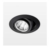
Recessed luminaire with LED, rated life of the LED L80/B10 50000 h (tambient 25°C), colour rendering index CRI > 80, chromaticity tolerance 2 SDCM (initial), rotation-symmetrical reflector with circular light distribution pattern, reflector pure aluminium 99,99% in MIRO-Silver®, segmented and faceted, 3D lens silicon to reduce the proportion of scattered light, die-cast aluminium, powder-coated, rotation angle, swivel angle +/- 25°, black,
