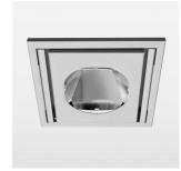
Recessed luminaire with LED, rated life of the LED L80/B10 > 50000 h, colour rendering index CRI > 80, chromaticity tolerance 2 SDCM (initial), reflector with circular light distribution pattern, reflector pure aluminium 99,99% in MIRO-Silver®,, swivel angle 30° luminaire housing sheet steel, powder-coated, silver, separate driver unit
