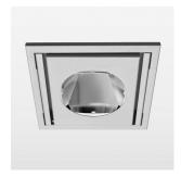
Recessed luminaire with LED, rated life of the LED L80/B10 > 50000 h, colour rendering index CRI > 80, chromaticity tolerance 2 SDCM (initial), reflector with circular light distribution pattern, swivel angle 30° luminaire housing sheet steel, powder-coated, silver, separate driver unit
