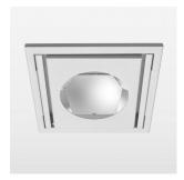
Recessed luminaire with LED, rated life of the LED L80/B10 > 50000 h, colour rendering index CRI > 90, chromaticity tolerance 2 SDCM (initial), reflector with oval light distribution pattern, swivel angle 30° luminaire housing sheet steel, powder-coated, white, separate driver unit
