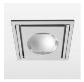
Recessed luminaire with LED, rated life of the LED L80/B10 > 50000 h, colour rendering index CRI > 70, chromaticity tolerance 2 SDCM (initial), reflector with oval light distribution pattern, swivel angle 30° luminaire housing sheet steel, powder-coated, silver, separate driver unit
