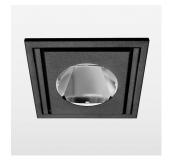
Recessed luminaire with LED, rated life of the LED L80/B10 > 50000 h, colour rendering index CRI > 82, chromaticity tolerance 2 SDCM (initial), reflector with circular light distribution pattern, reflector pure aluminium 99,99% in MIRO-Silver®,, swivel angle 30° luminaire housing sheet steel, powder-coated, black, separate driver unit
