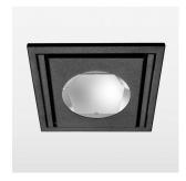
Recessed luminaire with LED, rated life of the LED L80/B10 > 50000 h, colour rendering index CRI > 70, chromaticity tolerance 2 SDCM (initial), reflector with oval light distribution pattern, swivel angle 30° luminaire housing sheet steel, powder-coated, black, separate driver unit
