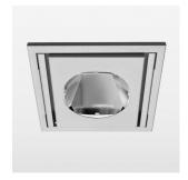
Recessed luminaire with LED, rated life of the LED L80/B10 > 50000 h, colour rendering index CRI > 90, chromaticity tolerance 2 SDCM (initial), reflector with circular light distribution pattern, reflector pure aluminium 99,99% in MIRO-Silver®,, swivel angle 30° luminaire housing sheet steel, powder-coated, silver, separate driver unit
