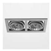
Recessed luminaire with LED, rated life of the LED L80/B10 > 50000 h, colour rendering index CRI > 90, chromaticity tolerance 2 SDCM (initial), reflector with circular light distribution pattern, swivel angle  $\pm$ 1-30° luminaire housing sheet steel, powder-coated, silver, separate driver unit
