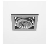
Recessed luminaire with LED, rated life of the LED L80/B10 > 50000 h, colour rendering index CRI > 90, chromaticity tolerance 2 SDCM (initial), reflector with circular light distribution pattern, reflector pure aluminium 99,99% in MIRO-Silver®, cardanic, swivel angle +/-30°, luminaire housing sheet steel, powder-coated, silver, separate driver unit
