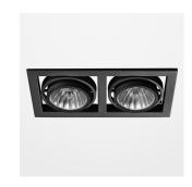
Recessed luminaire with LED, rated life of the LED L80/B10 > 50000 h, colour rendering index CRI > 90, chromaticity tolerance 2 SDCM (initial), reflector with circular light distribution pattern, swivel angle +/- 30° luminaire housing sheet steel, powder-coated, black, separate driver unit
