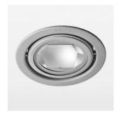
Recessed luminaire with LED, rated life of the LED L80/B10 > 50000 h, colour rendering index CRI > 80, chromaticity tolerance 2 SDCM (initial), reflector with circular light distribution pattern, reflector pure aluminium 99,99% in MIRO-Silver®, swivel angle +/-25°, luminaire housing sheet steel, powdercoated, silver, separate driver unit
