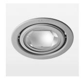
Recessed luminaire with LED, rated life of the LED L80/B10 > 50000 h, colour rendering index CRI > 90, chromaticity tolerance 2 SDCM (initial), reflector with circular light distribution pattern, reflector pure aluminium 99,99% in MIRO-Silver®, swivel angle +/-25°, luminaire housing sheet steel, powder-coated, silver, separate driver unit
