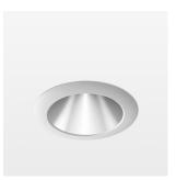
Recessed downlight with LED, rated life of the LED L80/B10 > 50000 h, colour rendering index CRI > 96, chromaticity tolerance 2 SDCM (initial), reflector with homogeneous light distribution pattern, diffuser lens, translucent, darklight reflector, aluminium, metallised, highgloss, luminaire head die-cast aluminium, powder-coated, ; mounting ring die-cast aluminum, front ring and coverblind plastic, white, separate driver unit
