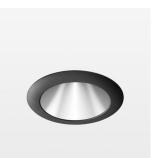
Recessed downlight with LED, rated life of the LED L80/B10 > 50000 h, colour rendering index CRI > 82, chromaticity tolerance 2 SDCM (initial), reflector with homogeneous light distribution pattern, diffuser lens, translucent, darklight reflector, aluminium, metallised, highgloss, luminaire head die-cast aluminium, powder-coated, ; mounting ring die-cast aluminum, front ring and coverblind plastic, black, separate driver unit
