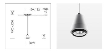
Suspended luminaire with LED, rated life of the LED L80/B10 > 50000 h, colour rendering index CRI > 96, chromaticity tolerance 2 SDCM (initial), reflector with circular light distribution pattern, reflector pure aluminium 99,99% in MIRO-Silver®,segmented and faceted, 3D lens silicon to reduce the proportion of scattered light, luminaire head die-cast aluminium, powder-coated, white, separate driver unit
