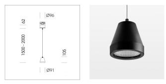
Suspended luminaire with LED, rated life of the LED L80/B10 > 50000 h, colour rendering index CRI > 90, chromaticity tolerance 2 SDCM (initial), reflector with circular light distribution pattern, reflector pure aluminium 99,99% in MIRO-Silver®,segmented and faceted, luminaire head die-cast aluminium, powder-coated, black
