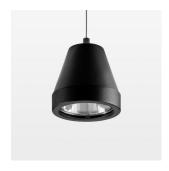
Suspended luminaire with LED, rated life of the LED L80/B10 > 50000 h, colour rendering index CRI > 90, chromaticity tolerance 2 SDCM (initial), rotation-symmetrical reflector with circular light distribution pattern, reflector pure aluminium 99,99% in MIRO-Silver®, segmented and faceted, 3D lens silicon to reduce the proportion of scattered light, luminaire head die-cast aluminium, powder-coated, black
