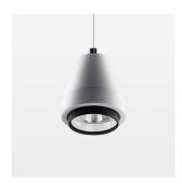
Suspended luminaire with LED, rated life of the LED L80/B10 > 50000 h, colour rendering index CRI > 90, chromaticity tolerance 2 SDCM (initial), reflector with circular light distribution pattern, reflector pure aluminium 99,99% in MIRO-Silver®, segmented and faceted, 3D lens silicon to reduce the proportion of scattered light, luminaire head die-cast aluminium, powder-coated, white
