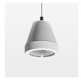
Suspended luminaire with LED, rated life of the LED L80/B10 > 50000 h, colour rendering index CRI > 96, chromaticity tolerance 2 SDCM (initial), reflector with circular light distribution pattern, reflector pure aluminium 99,99% in MIRO-Silver®, segmented and faceted, luminaire head die-cast aluminium, powder-coated, white
