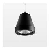
Suspended luminaire with LED, rated life of the LED L80/B10 > 50000 h, colour rendering index CRI > 90, chromaticity tolerance 3 SDCM (initial), rotation-symmetrical reflector with circular light distribution pattern, reflector pure aluminium 99,99% in MIRO-Silver®, segmented and faceted, 3D lens silicon to reduce the proportion of scattered light, luminaire head die-cast aluminium, powder-coated, black
