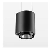
Suspended luminaire with LED, rated life of the LED L80/B10 50000 h (tambient 25°C), colour rendering index CRI > 95, chromaticity tolerance 2 SDCM (initial), reflector with circular light distribution pattern, 3D silicone lens to reduce the proportion of scattered light, reflector pure aluminium 99,99% in MIRO-Silver®, segmented and faceted, exchangeable reflector unit in high-sheen black plastic, with glass cover, luminaire housing die-cast aluminium, powder-coated, black
