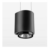
Suspended luminaire with LED, rated life of the LED L80/B10 50000 h (tambient 25°C), colour rendering index CRI > 90, chromaticity tolerance 2 SDCM (initial), reflector with circular light distribution pattern, 3D silicone lens to reduce the proportion of scattered light, reflector pure aluminium 99,99% in MIRO-Silver®, segmented and faceted, exchangeable reflector unit in high-sheen black plastic, with glass cover, luminaire housing die-cast aluminium, powder-coated, black
