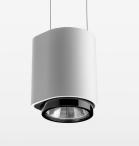
Suspended luminaire with LED, rated life of the LED L80/B10 50000 h (tambient 25°C), colour rendering index CRI > 82, chromaticity tolerance 2 SDCM (initial), reflector with oval light distribution pattern, 3D silicone lens to reduce the proportion of scattered light, reflector pure aluminium 99,99% in MIRO-Silver®, segmented, exchangeable reflector unit in high-sheen black plastic, with glass cover, luminaire housing die-cast aluminium, powder-coated, white
