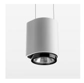
Suspended luminaire with LED, rated life of the LED L80/B10 50000 h (tambient 25°C), colour rendering index CRI > 80, chromaticity tolerance 2 SDCM (initial), reflector with circular light distribution pattern, reflector pure aluminium 99,99% in MIRO-Silver®, segmented and faceted, exchangeable reflector unit in high-sheen black plastic, with glass cover, luminaire housing die-cast aluminium, powder-coated, white
